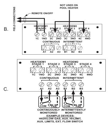
Figure 40 (A-C) - Terminal Strip Connection
